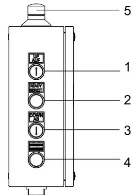
**Figure 14: Top platform control box, send/call configuration**
