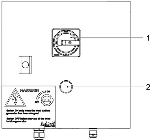
**Figure 11: Bottom platform control box, automatic send configuration with guard locking**
