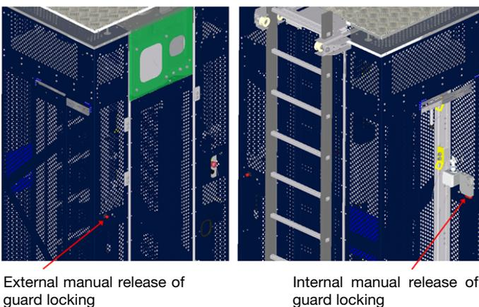
**Figure 6: Manual release of guard locking system**
