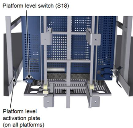
**Figure 5: Platform level switch**
