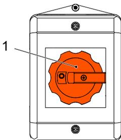
**Figure 12: Bottom platform control box, automatic send configuration for fences with trapped key or electrical switch monitoring system**
