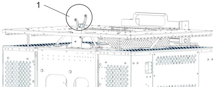
**Figure 19: Top limit and Emergency top limit switches**
