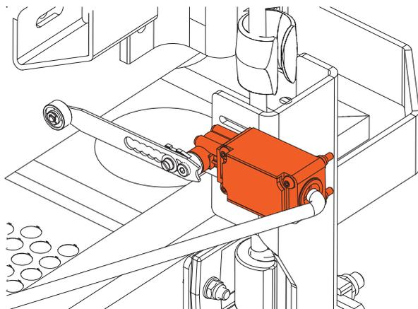
**Figure 24: Platform position switch**
