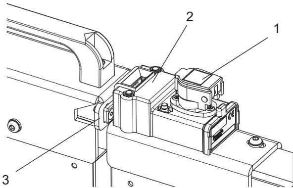
**Figure 23: Trapped-key system**
