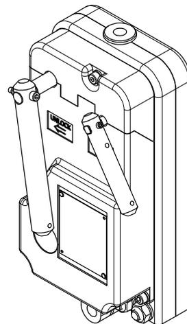
Figure 2 : Fall arrest device
