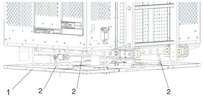
**Figure 20: Bottom obstruction device**
