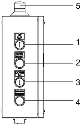
**Figure 15: Intermediate platform control box, send/call configuration**
