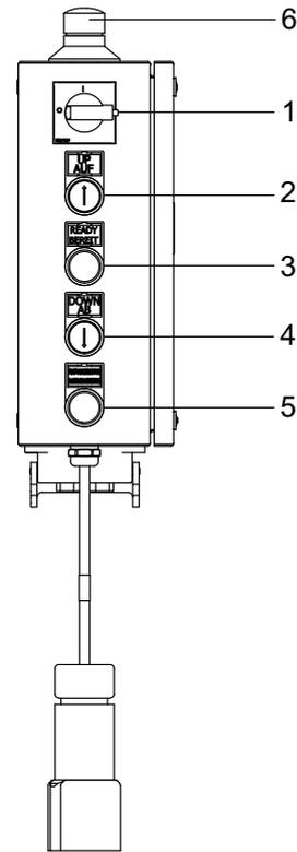
**Figure 13: Bottom platform control box, send/call configuration**
