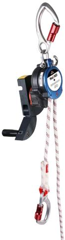
Device for rescuing or evacuating personnel from the Nacelle if the escape routes are blocked by fire. The device is fitted with a brake system that ensures that descending speed never exceeds 0.7m/sec (approx. half the normal walking speed). The low descend speed also helps to guarantee that the user has both hands free at all times. It is also approved for the descent of more than one person.
