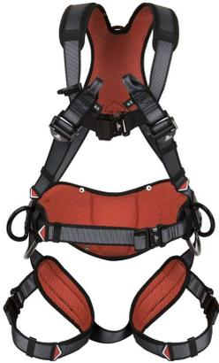
Comfortable, full-body harness with very lightweight back support, polyester strap material and D-rings. Approved for fall arrest, work positioning, rescue and evacuation. The harness has quick-lock buckles and a simple adjustment system on both front and back which makes it easily adaptable to individual needs/size. The front attachment makes the harness fit snugly against the torso when climbing.
